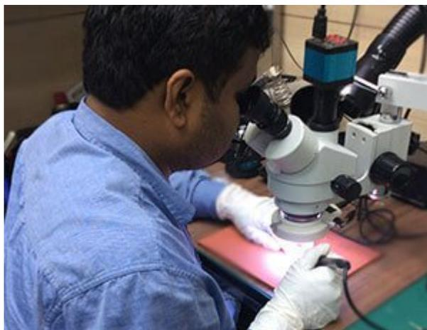
The engineers started cleaning/removing the coating from the chip. This is to check for data and controller signals in the memory card. We employed specialized data recovery tools to remove the coating from the memory card. We did this to test the functionality of the circuit board.
